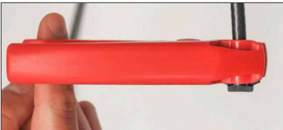
3. Insert the Series 6 coax into the appropriate wire strip tool so the end of the coax wire is flush against the outside of the tool.
