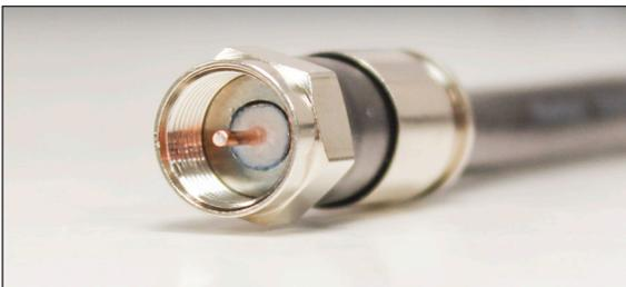
7. Gently press the Series 6 connector onto the coax cable. Ensure the Series 6 connector slides over the top of the aluminum foil layer. Pressing the fitting onto the coax with side-to-side motion. Keep pressing until the dielectric foam is flush with the inside of the Series 6 connector.
