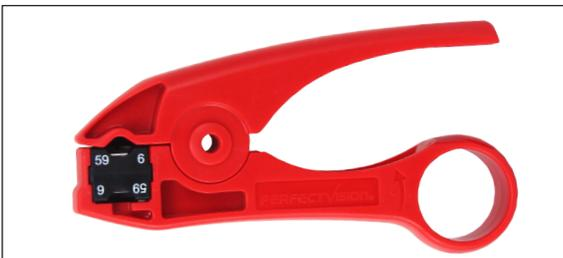
2. You must use the appropriate cable preparation tool for the specific cable you are installing. Quad cable, tri-shield, and standard dual shield Series 6 all use the same tool. The objective is to remove only the PVC coax jacket without damaging the underlying layer(s) of braid wire. It is imperative to use a SHARP blade in your cable preparation tool.
