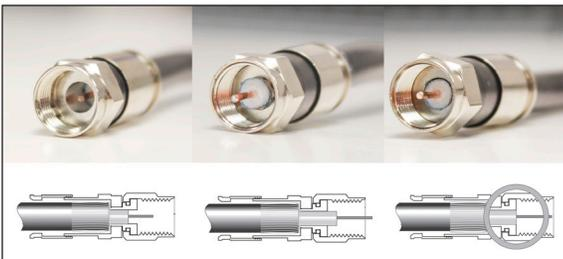
8. The fitting will slide down into the coax wire smoothly if you have aligned everything properly. Ensure that the white foam dielectric is in fact flush with the Series 6 connector. The Series 6 connector and cable should represent the image on the right. The image on the left is too short and the middle image is too far.
