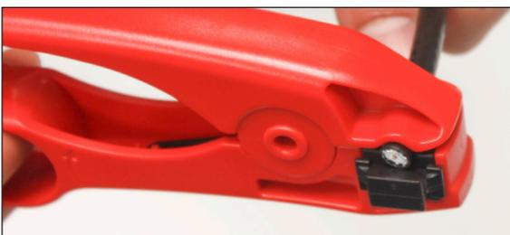
4. Turn the wire strip tool five or six full and continuous revolutions around the coax wire. Do not reverse the direction of the turn, it is unnecessary and can damage the braid.
