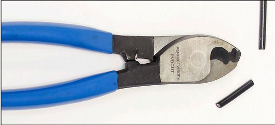
1. Cut the end of the Mini Series cable cleanly with sharp cutters at a 90° angle.
