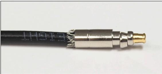
7. Gently press the Mini Series connector onto the coax cable. Ensure the connector slides over the top of the aluminum foil layer. Pressing the fitting onto the coax with a side-to-side motion.
