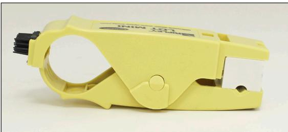
2. You must use the appropriate cable preparation tool for the specific cable you are installing. Quad cable, tri-shield, and standard dual shield Seris 6 all use the same tool. The objective is to remove only the PVC coax jacket without damaging the underlying layer(s) of braid wire. It is imperative to use a SHARP blade in your cable preparation tool.
