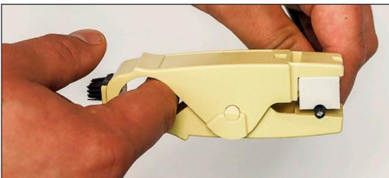
4. Turn the wire strip tool five or six full and continuous revolutions around the coax wire. Do not reverse the direction of the turn, it is unnecessary and can damage the braid.
