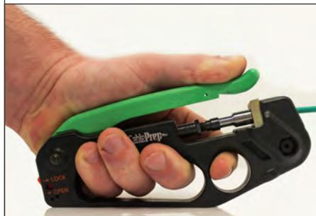
We recommend using the HPT6590WSMCPV compression tool. The tool is adjustable for various connector compression lengths. Our PVMCX requires a compression distance of 22.9mm.
