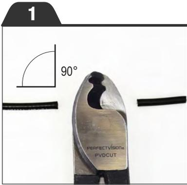
Cut the end of the cable cleanly with sharp cutters at a 90° angle.
